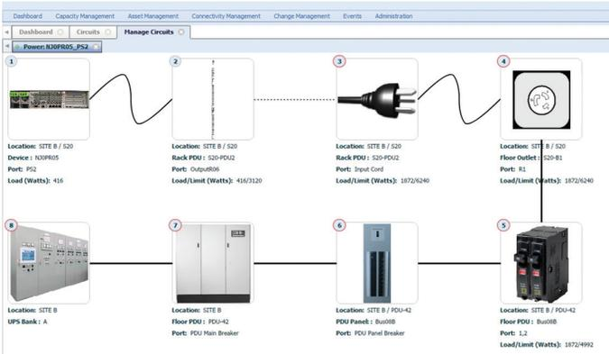
dcTrack provides the ability to budget power at every connection point from the UPS to the power supply with (n) or (N+1) redundancy.
