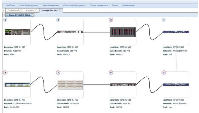
dcTrack allows you to build network connections with as few or as many hops possible.
